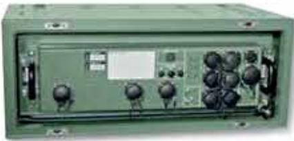
Housing with special anti-vibration frame
